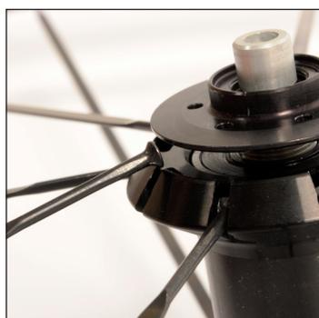
Insert each spoke head into the housings of one of the hub flanges, presenting them from the outside owing to the space freed up by the play in the axle. Repeat this operation for the other layer.
