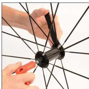
Insert the 5 mm Allen wrench into the end of the axle, side opposite the adjustment nut. Hold the adjustment nut with the hub wrench M40123.
