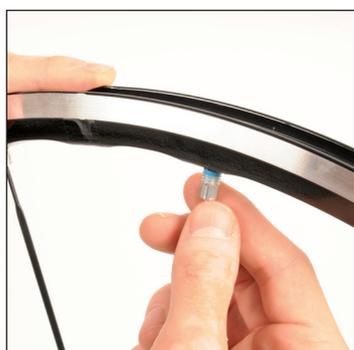
Manually pre-fit/screw in all the rim spokes until contact with the threadlocker.
