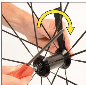
Using the Allen wrench and the hub wrench M40123, retighten the axle (counter-clockwise) until contact with the bearing is reached and then back off one-half turn.
