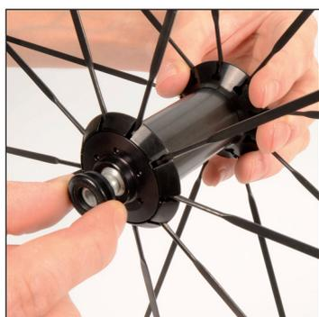
Adjustment nut side, remove the fork support which is clipped on the end of the axle.
