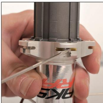
The 2nd spoke to the right of the valve hole is a non-traction spoke and will be on the inside: Insert it into the slot of the hub notch and do the same for every fourth spoke.
