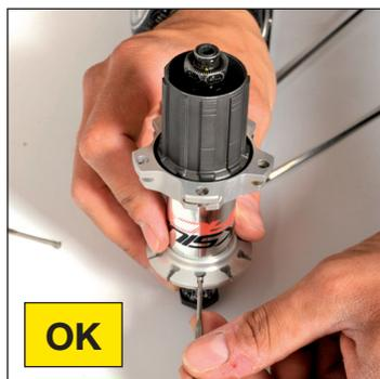
The first spoke on the non-drive side must be placed in a notch located opposite a notch on the drive side.
