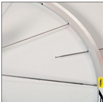
Turn the wheel over, then insert the remaining spokes (the longer ones) into the hub's remaining holes.
