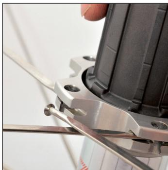
The 4th spoke to the right of the valve hole is a traction spoke and will be on the outside: Insert it into the slot of the hub notch and do the same for all the remaining spokes.
