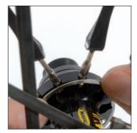
Replace the clip that holds the spokes in place and set the final tension and center the wheel taking care to respect appropriate spoke tensions.
