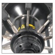
Fully unscrew the nipple to be replaced and remove it via the inside of the hub.
