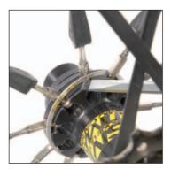
Turn the wheel on the drive side and remove the clip that holds the spokes in place using a small flat screwdriver.
