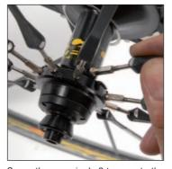
Screw the new nipple 2 turns onto the threaded rod and insert the nipple head into its correct position.
