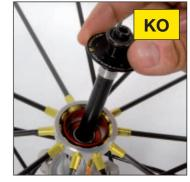
Without refitting the Tracomp ring, replace the axle so as to be able to place the wheel in the centering unit.
