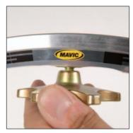
Screw the nipples into the rim using spoke wrench 996 079 01 until the thread lock has disappeared.
