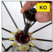
Without refitting the Tracomp ring, replace the axle so as to be able to place the wheel in the centering unit. Set the final tension and center the wheel taking care to respect appropriate spoke tensions.
