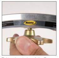
Tighten the nipples of the Tracomp spokes into the remaining rim holes until the thread lock disappears.
