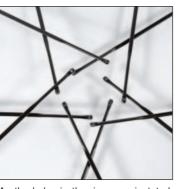
As the holes in the rim are orientated, the spokes are naturally positioned in the right direction. non-traction spokes must pass below the traction spokes, without touching at the crossover point.
