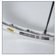
Screw the nipple of a Zicral spoke 2 turns into the 1st hole to the right of the valve hole, then do the same for all the Zicral spokes, 1 hole in 2 of the rim.
