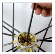
Turn the wheel over and insert all the Tracomp spokes, nipple first, into the hub on the non-drive side.
