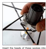
the hub slots: the heads of these spokes into the hub slots: the heads of the nontraction spokes should be inserted into the inside slits of the slots, the heads of the traction spokes into the outside slits.
