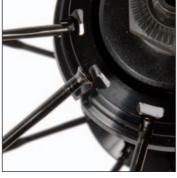
Introduce the head of each spoke into the receiving positions on one of the hub's flanges:
