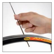
Prepare the spokes by screwing a nipple 3 turns onto each, and then thread the spokes, head first, into every other hole of the rim, from the outside.
