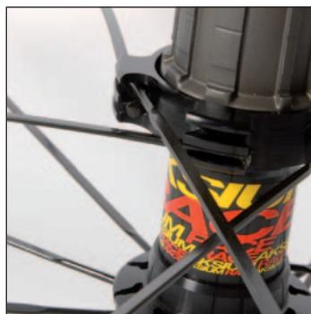
The 3rd spoke to the right of the valve hole is a traction spoke: insert it into an outside notch of the hub and repeat this for all the remaining spokes.
