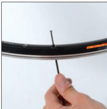
With the valve hole near you, thread a spoke, head first, into the first hole to the right of the valve hole, and continue every 1 hole in 2.
