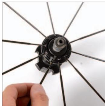
Introduce the head of each spoke into the receiving positions on the hub's flange, on the non-drive side, from the outside of the flange.
