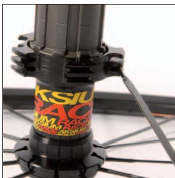
The first spoke to the right of the valve hole is a non-traction spoke: insert it into an inside notch of the hub and repeat this 1 spoke out of 4.
