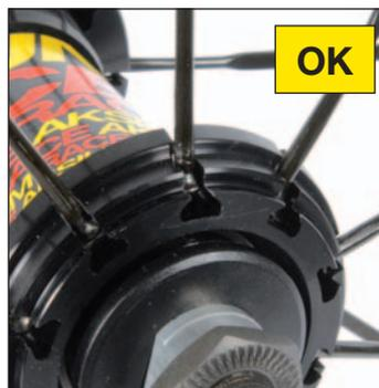
Screw each nipple uniformly (1 turn of the spoke wrench for each spoke and for each turn of the wheel) to tension the wheel, checking the heads are correctly positioned in the groove of the hub on the non-drive side to ensure a spoke does not become unhooked and to prevent the hub from breaking.
