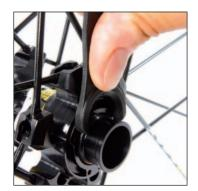
Introduce end lugs of the hub wrench M40123 into the holes of the adjustment nut on the non-disc side.
