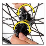
Refit the axle by tightening the adjustment screw as far as possible and then unscrew it 1/4 of a turn.
