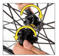
Manually keep the axle on the disc side in place and fully unscrew the adjustment nut using the hub wrench. Remove the hub axle.
