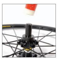
Use the bearing press kit M40218 to remove the old bearings and fit the new ones.
