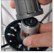
Fit the spacer washer to the hub body bearing, lower the pawls and refit the free wheel body to the hub.
