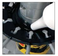
Lubricate the toothed area inside the free wheel body such that 2 to 3 grooves of the free wheel body are filled. Also place a drop of Mavic mineral oil M40122 on the seal lip.
