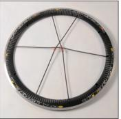
Fit the third spoke in the ninth hole to the right of the valve hole, counting counter-clockwise. The other end of this spoke is inserted in the nineteenth hole.
