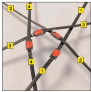
The fourth spoke is inserted in the thirteenth hole and must pass above the second and third spokes then underneath the first. Its other end is inserted in the third hole.
