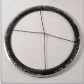
Fit the second spoke in the fifth hole to the right of the valve hole, counting counter-clockwise. The other end of this spoke is inserted in the fifteenth hole.
