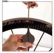
Adjust the wheel definitively by holding the spoke heads inside the carbon rim flange with holding tool 101 295 01.
