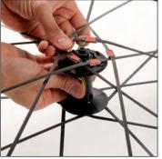
Offer up the hub in the middle of the spokes and position the two hub flanges between the two layers of spokes.
