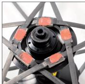
Position the plates in the housing on one side of the hub then the other.
