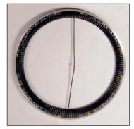
With the valve hole near you, screw a spoke in the first hole to the right of the valve hole and its other end in the eleventh hole when counting clockwise.
