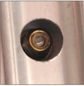
Turn the wheel over and repeat the steps above. Tighten all nipples until the threaded rods are just brushing the nipples.
