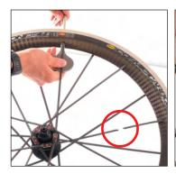
and loosen both ends of the spoke pair which passes over the spoke pair to be replaced in the hub flange perimeter.
