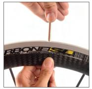
holding the spoke heads with the thumb the spoke heads inside the carbon rim across the carbon rim flange.
