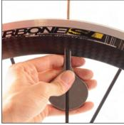
Retension the two spoke pairs involved, Adjust the wheel definitively by holding flange with holding tool 101 295 01. This tool should be offered up via the side with the most space and must enter without forcing.
