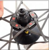
Mark the spoke pair you wish to replace Remove the old spoke pair and fit the new one in place in the hub, respecting the original lacing.
