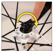
Refit the adjustment nut and the frame support.
