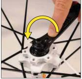
Completely unscrew the adjustment nut with the hub wrench 325 423 01.
