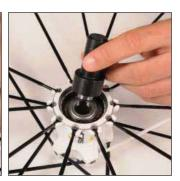
Position the drive side bearing with the disc side bearing seal. Refit the bearing with press kit M40119.
