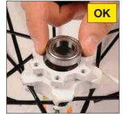
In order to ensure a perfect seal of the free wheel mechanism, the bearings of the hub body must be mounted with the disc side seal.
