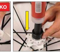
Fit the new non-drive side bearing with press kit M40119.
