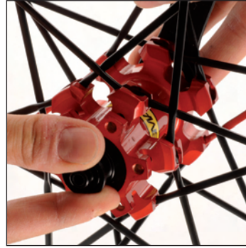
Refit the axle by inserting it in the hub via the disc side and retighten the adjustment nut with the hub wrench with your fingers.
