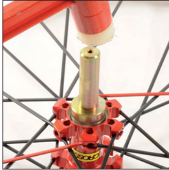
Fit the new bearings with press kit 996 887 01.
