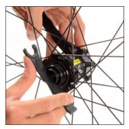
Retighten the adjustment nut with the hub wrench, holding the axle by hand (Crossmax SX) or with the handle of a second wrench M40123 inserted in the axle slits (Crossline) until contact is made with the bearing and loosen it again by a quarter turn.
