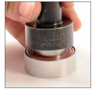
If the non-disc side spacer has come out of the hub during removal, start by fitting the new bearing to the spacer with press kit M40218.
