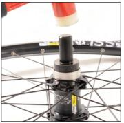
Refit the bearings-spacer assembly in the non-disc side hub, pushing it home with press kit M40218.
