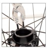
Refit the circlip via the non-disc side with the circlip clamp.
