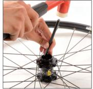
Remove the disc side bearing by pushing it from outside the hub with a press kit to extract the bearing from the other side.
