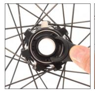
Insert the end lugs of hub wrench M40123 in two offset holes in the adjustment nut on the non-disc side.
