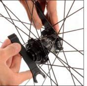
Hold wrench M40123 in place and loosen the axle via the disc side with your fingers (Crossmax SX) or the handle of a second wrench M40123 inserted in the axle slits (Crossline).
