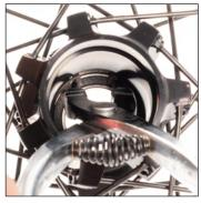
Remove the circlip via the non-disc side bearing by with the circlip clamp. Remove the disc side bearing by pushing it from outside the hub w
