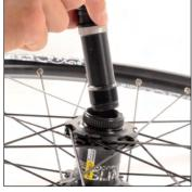
Insert the axle in the hub via the disc side. For the Crossmax SX 09, make sure that the shim washer is fitted.
