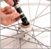
Remove the axle. Take care on the Crossmax SX not to mislay the bearing shim washer slid onto the axle.
