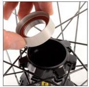
Remove the non-disc side bearing. As the bearing is fitted in a spacer, this could be removed with the bearing. You must therefore separate the spacer from the bearing.
