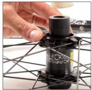
Insert the new disc side bearing via the non-disc side and push it home with press kit M40218 and an additional tube.
