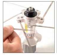
Offer up the head of a driving spoke passing underneath the rim, underneath the first non-driving spoke then over the second non-driving spoke. Insert the head of this spoke in the notch in the corresponding slot.
