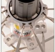
Turn the wheel over, screw a (short) spoke in all the remaining holes in the rim then push their heads in the slots on the drive side hub.
