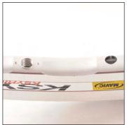
Turn the rim so that the two raised indicator bumps are to the left of the valve hole when this is near you.
