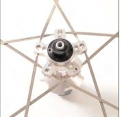
Tighten the nipple on this spoke in the corresponding hole on the rim, then do the same for all the non-drive side driving spokes.
