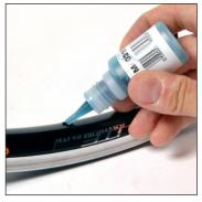
Start by placing a drop of Mavic thread lock M40315 in each threaded hole on the rim.
