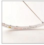
Screw a spoke in the third hole to the right of the valve hole until the nipple locks. Repeat this step for all the spokes, one hole in four on the rim.
