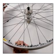
Tighten the nipple on a **non-driving** spoke (outside section of a slot to the left of the hub axle) until it locks in the third hole to the right of the valve hole.
