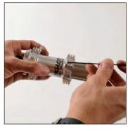
Offer up the head of a spoke to a slot, keeping it parallel to the hub axle, via the outside of the wheel.
