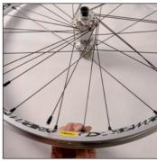
Tighten the nipple on a **driving** spoke (inside section of a slot to the right of the hub axle) until it locks in the **first** hole to the right of the valve hole.
