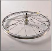
Turn the wheel over and insert all the non-drive side spokes using the procedures detailed in the first four steps above.
