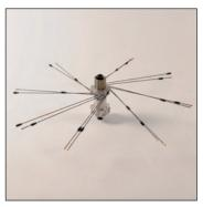
Fit all the drive side spokes in this way. Turning them all in the same direction will make it easier to fit the remaining spokes.
