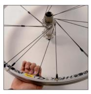
Tighten the nipple on a **non-driving** spoke (**inside** section of a slot to the right of the hub axle) until it locks in the **first** hole to the right of the valve hole.
