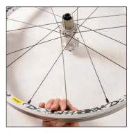
Tighten the nipple on a **driving** spoke (**outside** section of a slot to the left of the hub axle) until it locks in the **third** hole to the right of the valve hole.
