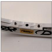
With the valve hole near you, turn the rim so that the raised indicator bumps are to the right of the valve hole.
