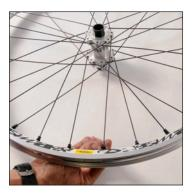
Tighten the nipple on a **braking** spoke (**outside** section of a slot to the right of the hub axle) until it locks in the **first** hole to the right of the valve hole.
