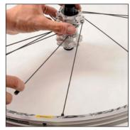
Repeat these steps for all the **non-braking** spokes inserted in the **inside** sections of slots, one hole in four in the rim.
