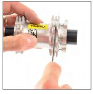
Slide this spoke in the outside section of the slot and lower it tangentially to the hub.
