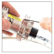
Offer up the head of a spoke to a slot, keeping it parallel to the hub axle, via the outside of the wheel.
