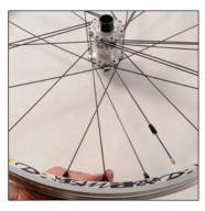
Tighten the nipple on a **non-braking** spoke (**inside** section of a slot to the left of the hub axle) until it locks in the **third** hole to the right of the valve hole.
