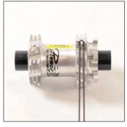
Fit all the disc side spokes in this way. Turning them all in the same direction will make it easier to fit the remaining spokes.
