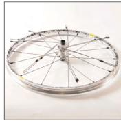
Turn the wheel over and insert all the non-disc side spokes using the procedures detailed in the first four steps above.
