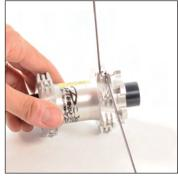
Repeat the operation with a new spoke in the same slot, but this time for the inside section of the slot.
