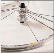
Tighten the nipple on a **non-braking** spoke (**inside** section of a slot to the right of the hub axle) until it locks in the **first** hole to the right of the valve hole.
