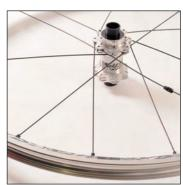
Tighten the nipple on a **braking** spoke (**outside** section of a slot to the left of the hub axle) until it locks in the **third** hole to the right of the valve hole. Repeat these steps for all the **braking** spokes inserted in the **outside** sections of slots, one hole in four in the rim.
