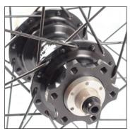
The doglegs on the driving spokes on the non-drive side of the rear wheel must be facing towards the inside of the hub flange.
