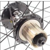
The doglegs on the driving spokes on the drive side of the rear wheel must be facing towards the outside of the hub flange.
