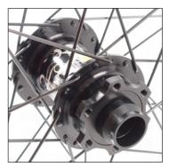
The doglegs on the braking spokes on both sides of the front wheel must be facing towards the outside of the hub flanges.
