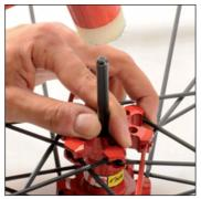
Use the bearing press kit to remove the bearings.
