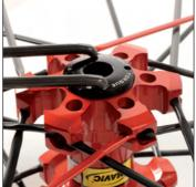
Refit the bearing protection cap with the hub wrench (9 Nm torque).
