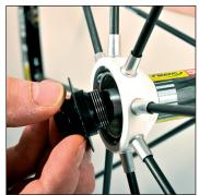
Select the fork support optimizing the play adjustment using the QRM SL bearing play adjustment procedure.
