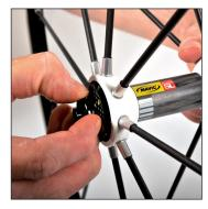
By hand, remove the fork support Push (clipped onto the axle) from the label side hub. of the hub.
