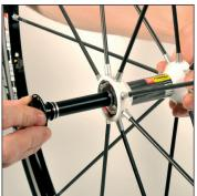
Introduce the axle into the side opposite the hub label.
