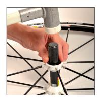
Use the bearing kit to fit the bearings 323 909 01.
