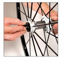
By hand, remove the frame support (clipped onto the axle) from non-drive side.
