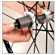
Remove the axle by pushing on the screw at the end of the axle, drive side.
