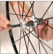
Fit the 5 mm Allen wrench in the axle on the drive side and the 10 mm Allen wrench on the non-drive side. Unscrew the axle.
