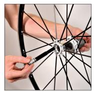
Refit the new axle (tightening torque 15 Nm).
