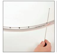
With the valve hole near you, insert a spoke head first into the second hole to the right of the valve hole, then continue with every second hole.
