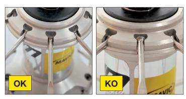
Screw each of the nipples uniformly (1 spoke wrench turn for each spoke and per wheel turn) to tension the wheel, <u>while checking the proper position of their head</u> <u>in the bottom of the hub groove</u> to prevent spoke displacement or hub breakage.
