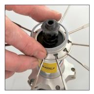
Clip the hub cap on the hub flange. (This will help you to keep the spokes in place during this operation)
