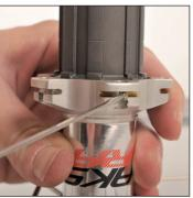
The 2nd spoke to the right of the valve hole is a non-traction spoke and will be on the inside: Insert it into the slot of the hub notch and do the same for every fourth spoke.
