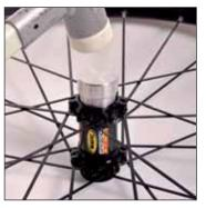
Using press bearing kit 996 887 01, fit the new non-disc side bearing.
