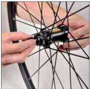
Remove the axle from the disc side.
