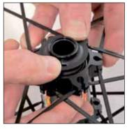
Replace the dust cover by pushing it parallel to the axle.
