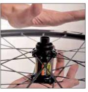
Remove the tapered washer, the pin and flat washer by taping gently on the axle, disc side (Caution: be careful not lose these 3 elements!).
