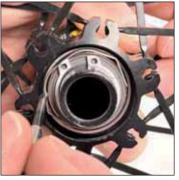
Maintain pressure on the axle, on the non-disc side, and simultaneously press on the pin at 3 points with a screwdriver (2 at the end + center) to slide it inside.
