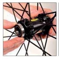
Insert the new disc side bearing via the non-disc side and push it home with press kit 996 887 01.
