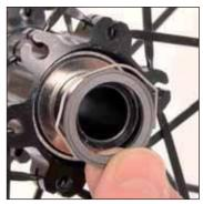
Mount the pin / washer assembly on the non-disc side by presenting the conical part toward the inside, and the grooved part toward the outside.
