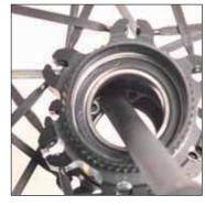
Insert the bearing press from the disc side and remove the non-disc side bearing to the outside (be careful not to damage the circlip near the bearing).
