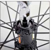
Remove the circlip using an external circlip pliers.
