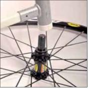
From the disc side, using the bearing press 108 850 01, remove the disc side bearing toward the outside.
