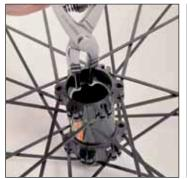
From the non-disc side, using an interior circlip pliers, remove the first interior circlip (non-disc side) then the second interior circlip (disc side).
