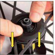
Place your thumbs on the two opposite edges of the cap and press to clip the cap onto the hub body.
