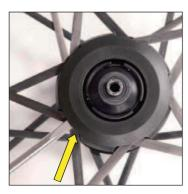
Insert a flat-tip screwdriver (ideally 5 x 125 mm) fully into an opening at the junction of two spokes. The tip of the screwdriver should be against the hub body.
