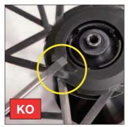
Caution: the screwdriver must be correctly positioned between two spokes and be in contact with the hub body. Incorrect positioning may result in spoke damage.
