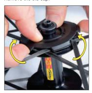
Unclip and remove the old hub cap by pressing on the inside with your thumbs while lifting the outside with your fingers.
