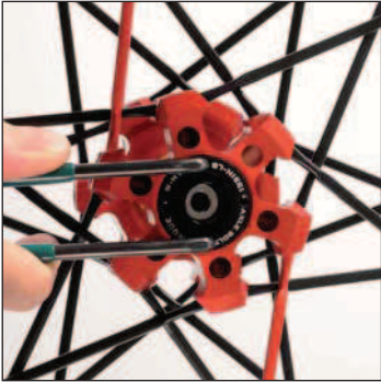
Loosen the non-disc side bearing protection cap with the hub wrench.
