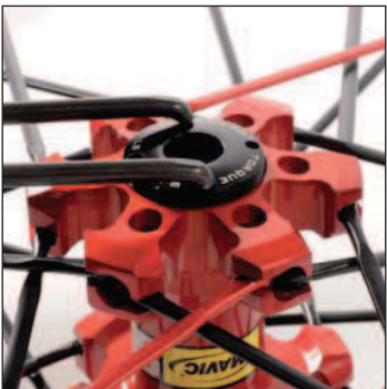
Refit the bearing protection cap with the hub wrench (9 Nm torque).
