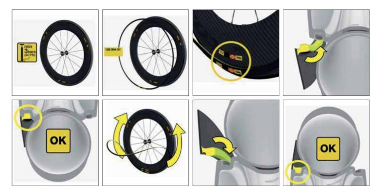
Repeat the operation for the 2nd blade, then inflate to the desired pressure (6 to 11 bar).
