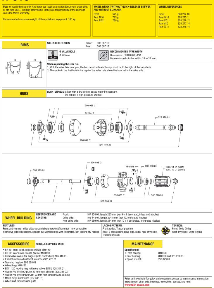
Never turn a Tracomp spoke nipple without having first removed the Tracomp rings from the hub, otherwise the spoke may be irreversibly damaged. Never fit a computer magnet other than the one supplied with the wheel. Only transport the wheels in the wheel bags supplied. Avoid side shocks to the Tracomp spokes.
