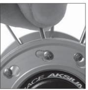
Pass the elbowed part of each spoke through the slot in the hub flange.
