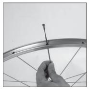
Prepare the spokes by screwing a nipple onto each spoke until it locks, then thread the spokes, elbow first, into each rim hole from the outside.
