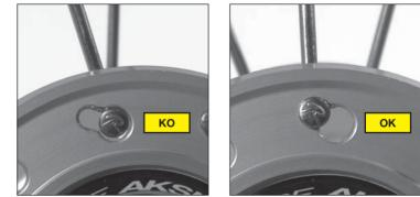
Re-tighten the spokes to the correct wheel tension ensuring that the head of each spoke is correctly positioned.
