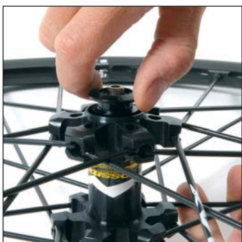
Hand screw the adjustment nut and keep it in place using the hub wrench M40123.
