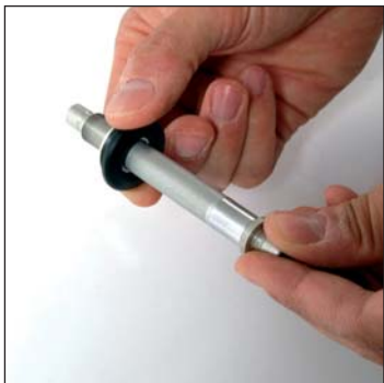
If the bearing cover needs replacing, slide it along the axle to remove it.
