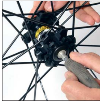
Insert the 5 mm Allen wrench into the axle, on the opposite side to the adjustment nut, and unscrew it.
