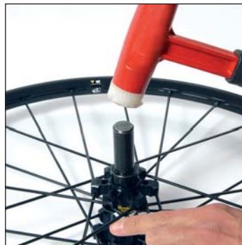
Use the bearing press kit M40120 or M40373 to fit the new bearings.
