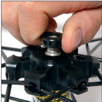
Unclip the fork support nuts from each side of the hub.
