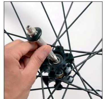
Refit the bearing cover onto the axle and then replace the axle into the hub from the disc side.
