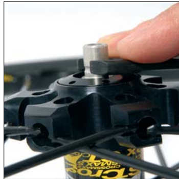
Block the adjustment nut using the hub wrench M40123.
