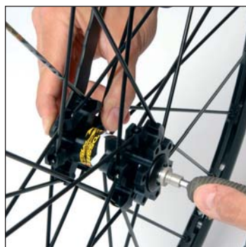
Insert the 5 mm Allen wrench in the opposite side to the adjustment nut, screw until the stop is reached and then unscrew it by 1 turn.
