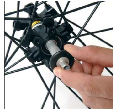
Unscrew the adjustment nut completely and remove the axle from the hub.
