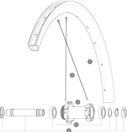
RIMS : 1 V4090410 KIT FRONT RIM KSYRIUM PRO CARBON UST DISC TdF 20 / KSYRIUM P V2620101 UST RIM TAPE 25mm (for 21-24mm wide rim) **SPOKES** 2 V3666301 KIT 12 FRT/NDS BUTTED AERO STAINLESS SPOKE 283 KSYRIUM PRO C **HUB SHELLS** N/A 3 HUB BODY 4 V2500901 KIT BEARINGS 18x30x7 + WAVED WASHER + CLIP V2374101 KIT QRM AUTO FRONT L3 AXLE 100x12mm DCL - while stock last 5 5 V2374001 KIT 12x100mm FRONT AXLE DCL QRM AUTO ALLROAD > 2019 **ADAPTERS** V2680301 "Kit Ft Road Adapter 12 >> 9mm"
